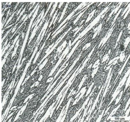
CORODUR-79 Photomicrograph 1 Primary Carbides
